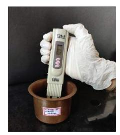
Figure 3: TDS value of water is 429 ppm in copper vessel. TDS: Total dissolved solutes
