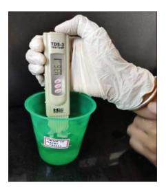
Figure 4: TDS value of water is 436 ppm in plastic vessel. TDS: Total dissolved solutes
