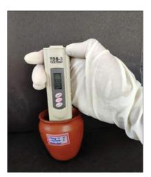
**Figure 16:** TDS value of water is 208 ppm after addition of *Nimba Patra Churna* in clay vessel. TDS: Total dissolved solutes
