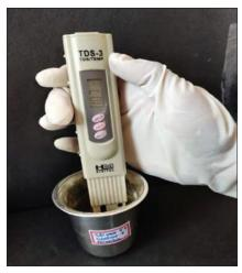
**Figure 12:** TDS value of water is 107 ppm after addition of *Nimba Patra Churna* in silver vessel. TDS: Total dissolved solutes
