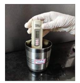
Figure 5: TDS value of water is 445 ppm in steel vessel. TDS: Total dissolved solutes
