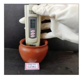
Figure 26: TDS value of water is 169 ppm after addition of *Kataka Beeja Churna* in clay. TDS: Total dissolved solutes
