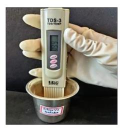
**Figure 22:** TDS value of water is 199 ppm after addition of *Kataka Beeja Churna* in silver vessel. TDS: Total dissolved solutes
