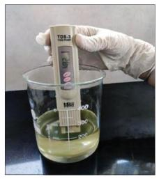
Figure 1: TDS value is 482 ppm of sample water. TDS: Total dissolved solutes
