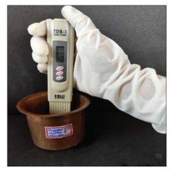
**Figure 13:** TDS value of water is 157 ppm after addition of *Nimba Patra Churna* in copper vessel. TDS: Total dissolved solutes
