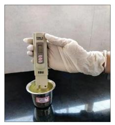
Figure 2: TDS value of water is 372 ppm in silver vessel. TDS: Total dissolved solutes
