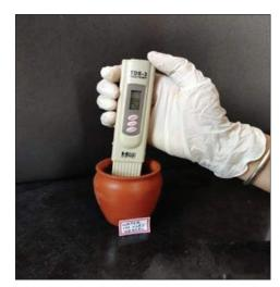
Figure 6: TDS value of water is 628 ppm in clayvessel. TDS: Total dissolved solutes
