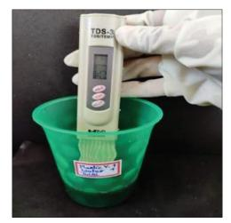
**Figure 19:** TDS value of water is 257 ppm after addition of *Tulsi Patra Churna* in plastic vessel. TDS: Total dissolved solutes
